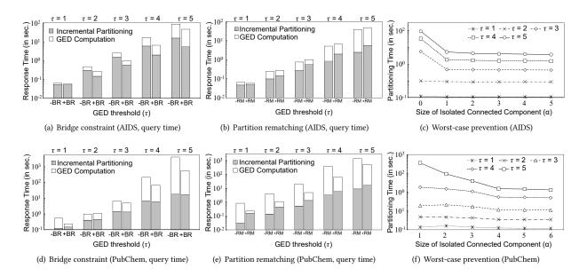
Figure 9: Evaluating optimization methods in Inves incremental partitioning
