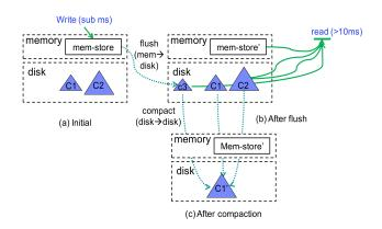
Figure 2: Log Structured Merge tree.
