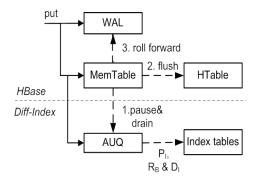
Figure 5: Recovery process of AUQ.
