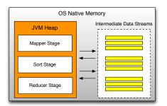
Figure 5: Offloading intermediate data to off-heap direct native memory.
