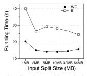
Figure 8: Running time of word count and inverted indexing on the 512MB dataset with different split sizes (running 16 threads).
